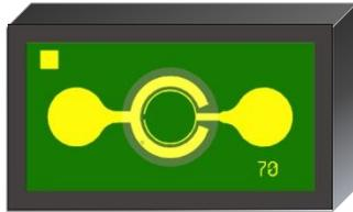
This product is a high-performance front side illuminated InGaAs PIN photodiode chip that features low capacitance, high responsivity, low dark current and excellent reliability. This product has a large 70 $\mu$ m detection window, and is intended primarily to be integrated with a pre-amplifier in a hermetic TO package, designed to meet performance requirements for data rates up to 4.25Gbps data communication over single-mode optical fiber at 1200nm to 1600nm.
